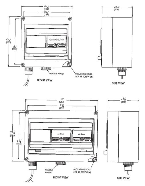
$^{\star}$  For complete dimensions, see WT.050.130.100 for single point, WT.050.130.102 for dual point, and WT.050.130.104 for battery backup.b
