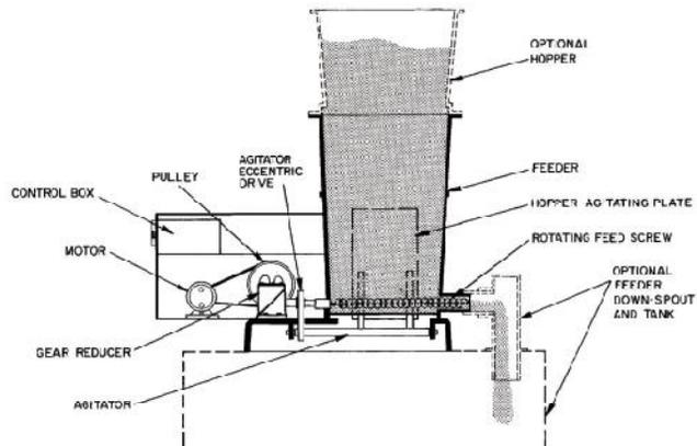
A float valve, dust-and-fume arrester, and mechanical mixer can be added to the tanks. Also available are packaged feeder-solution tank systems with 6 tank sizes from 35 to 500 gallons (see page 6). A complete line of hopping components includes bag loaders, dust collectors, and hoppers in many styles and sizes along with accessories and installation hardware. The feeder hopper is designed to support up to 1000 lb.
